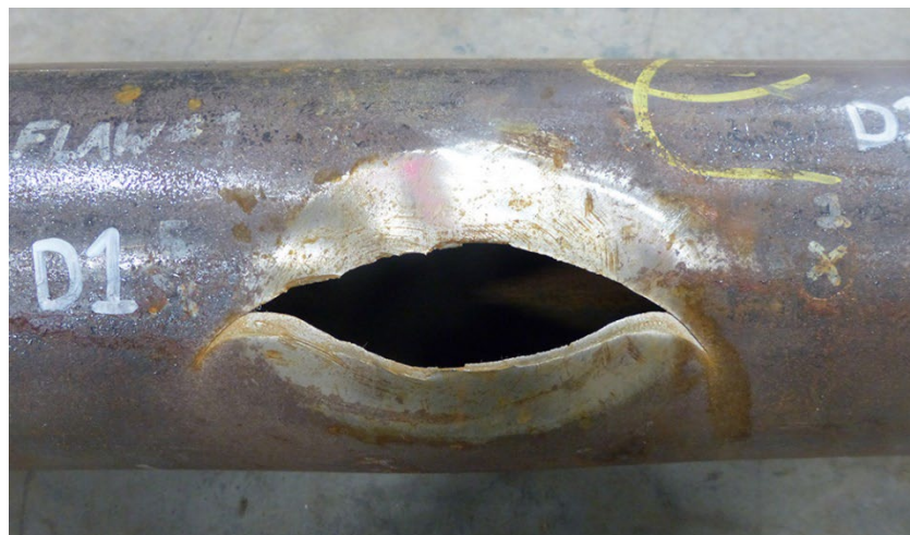
Figure E.44 – Failed Specimen (5.5in-JT#3-D1)
