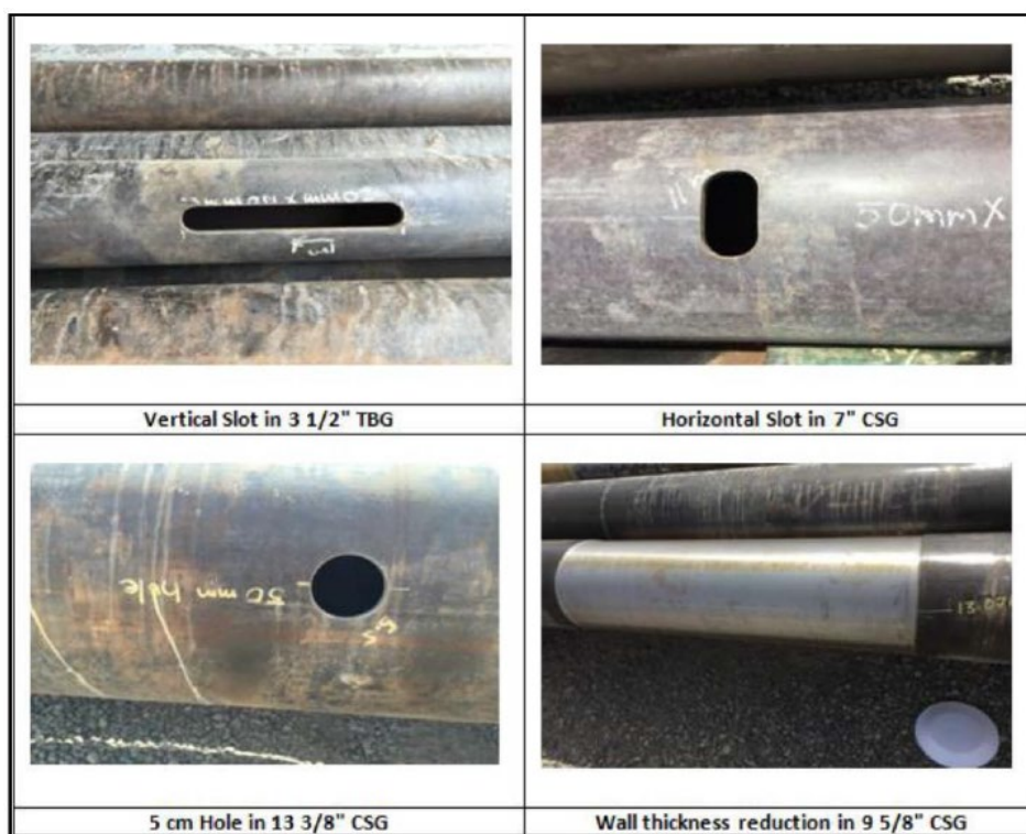
Figure 6 – Examples of Machined Features in PDO Test Program [15]
