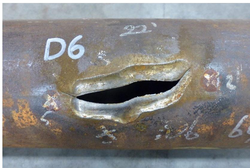
Figure E.29 – Failed Specimen (4.5in-JT#3-D6)
