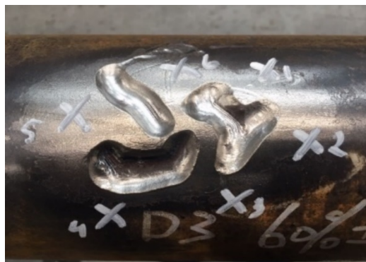
Figure 13 – Random Shape Metal Loss Feature Example (4.5in-JT#3-D3)
