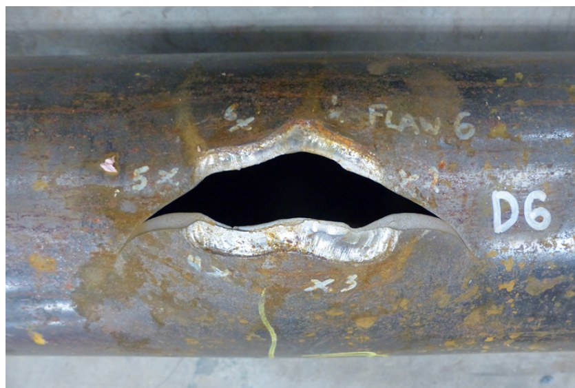
Figure E.99 – Failed Specimen (7.0in-JT#3-D6)
