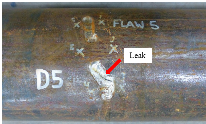
Figure E.94 – Failed Specimen (7.0in-JT#3-D5)
