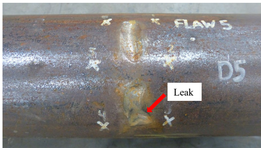
Figure E.64 – Failed Specimen (5.5in-JT#3-D5)
