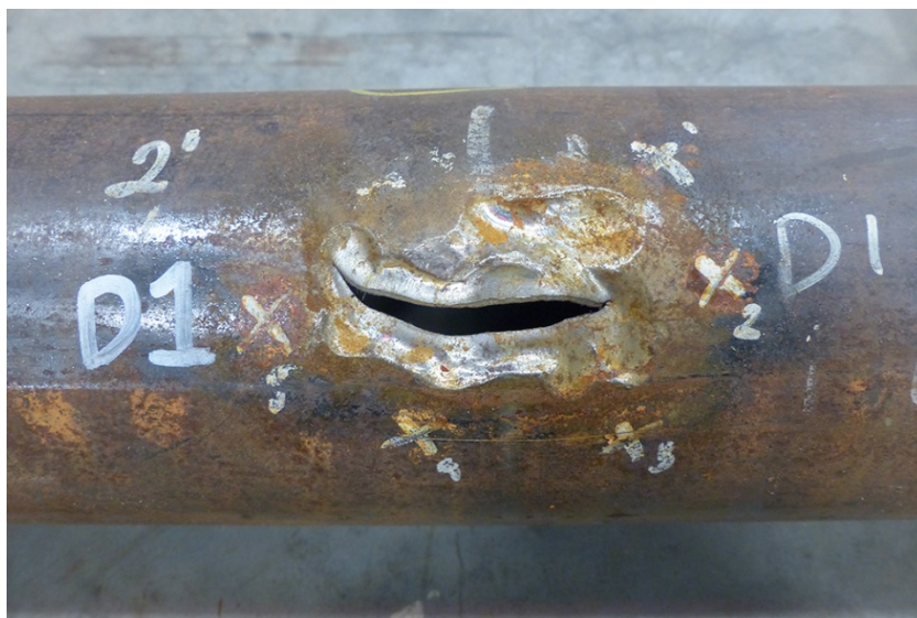
Figure E.4 – Failed Specimen (4.5in-JT#3-D1)
