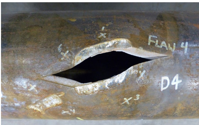
Figure E.89 – Failed Specimen (7.0in-JT#3-D4)
