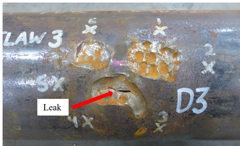
Figure E.54 – Failed Specimen (5.5in-JT#3-D3)
