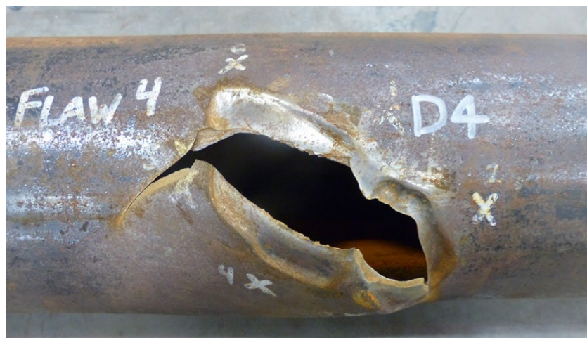
Figure E.59 – Failed Specimen (5.5in-JT#3-D4)
