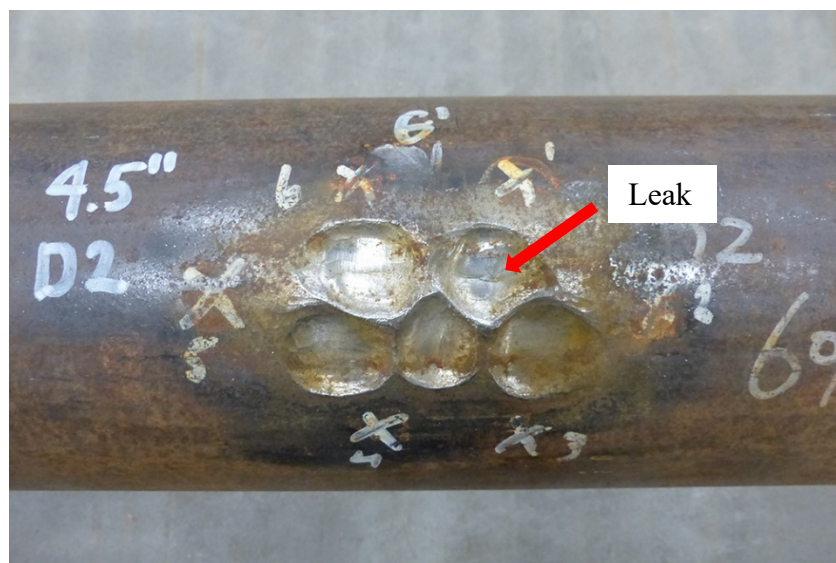
Figure E.9 – Failed Specimen (4.5in-JT#3-D2)
