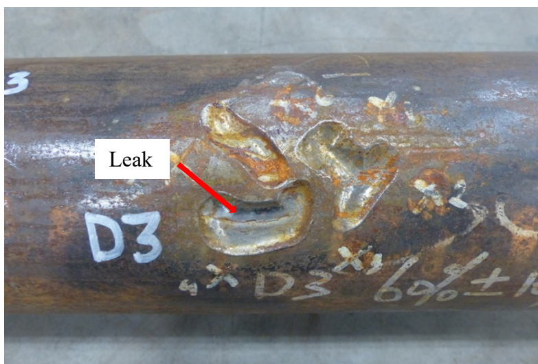
Figure E.14 – Failed Specimen (4.5in-JT#3-D3)
