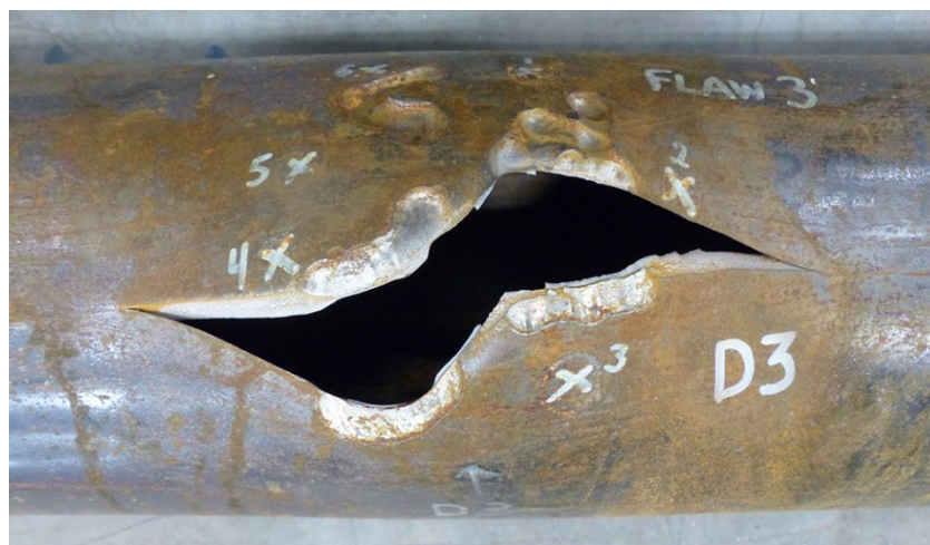
Figure E.84 – Failed Specimen (7.0in-JT#3-D3)
