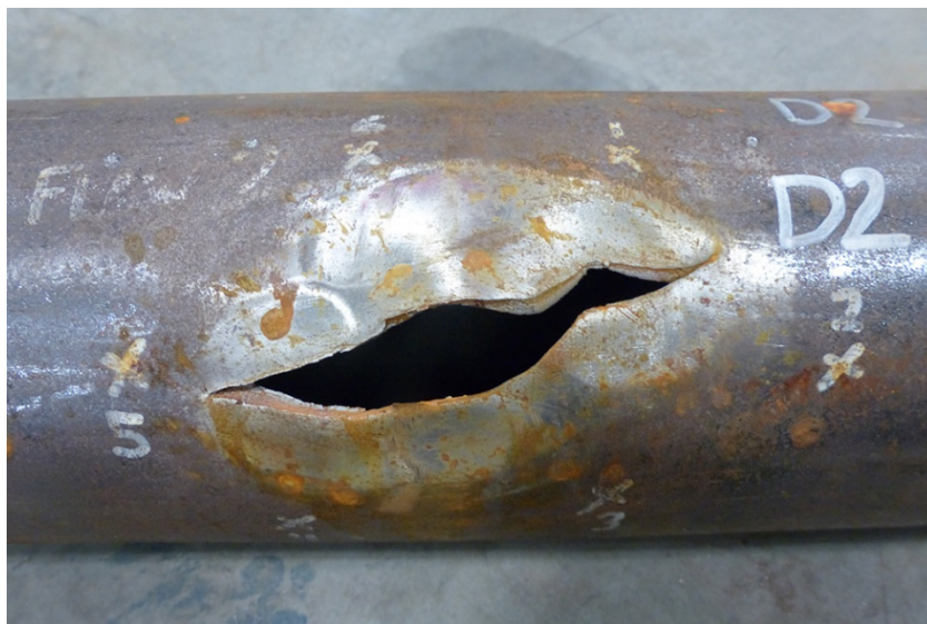
Figure E.49 – Failed Specimen (5.5in-JT#3-D2)
